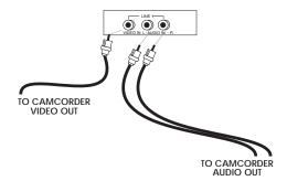
For added convenience when you want to connect video equipment to your 8mm/VHS Dual-Deck VCR temporarily, use the Line 1 Video and Audio input jacks located on the front of your 8mm/VHS Dual-Deck VCR. The Line 1 jacks work just the same as the Line 2 jacks on the back of the VCR. Simply select LINE 1 instead of LINE 2 for TV VIEW and as the RECORD SOURCE in the VHS MENU.
